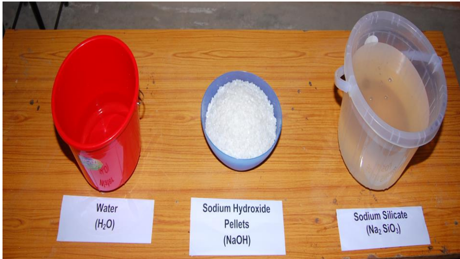
Fig. 3 Preparation of Alkaline Activator Solution
