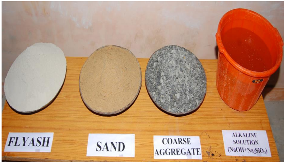
Fig. 4 Constituents of Geopolymer Concrete
