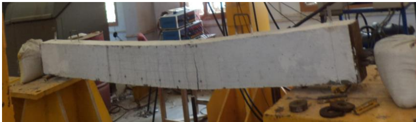
Fig. 39 Crack Pattern of GPC Post Tensioned Beam
