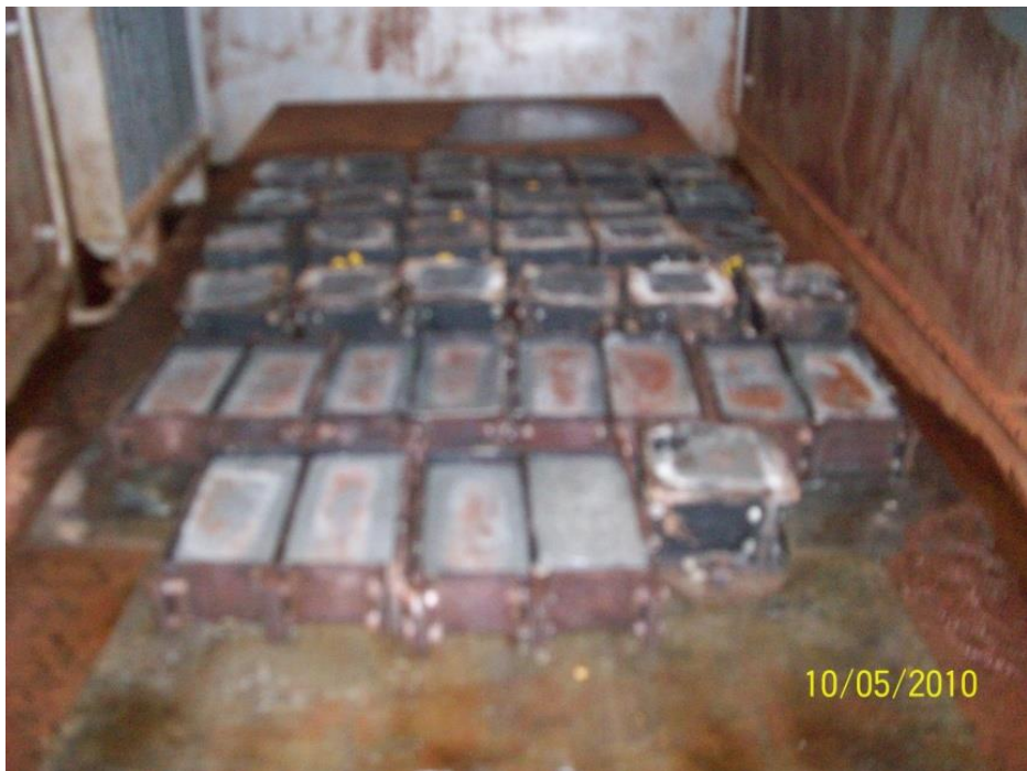
Fig. 15 Steam Curing of Geopolymer Bricks
