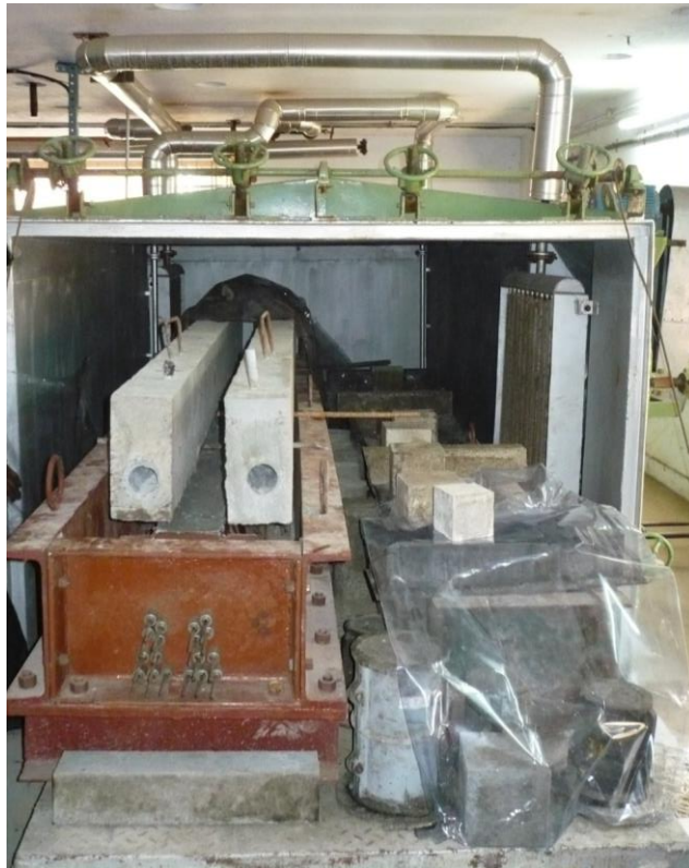
Fig.35 Specimens kept in Steam Curing Chamber
