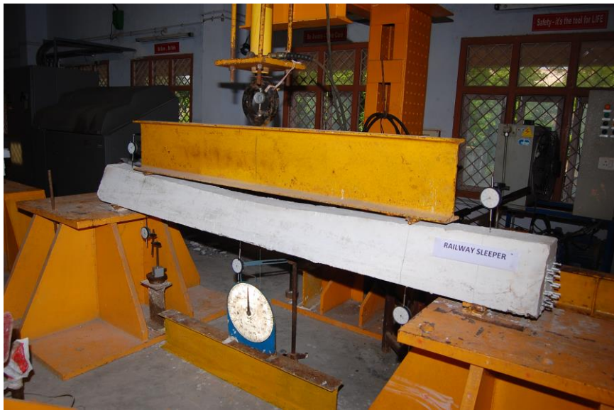
Fig. 29 Experimental Setup of the Sleeper (GPC)
