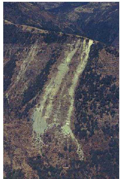
Huge landslides extending many hundreds of metres, in both forested and deforested slopes. Roads are cut with little thought to slope stabilisation. Given the very loose soil even the presence of trees does not always guarantee soil stability. Above: slides along a small track in Eaglenest sanctuary. Below: slides along the highway in Dirang and Jang.
