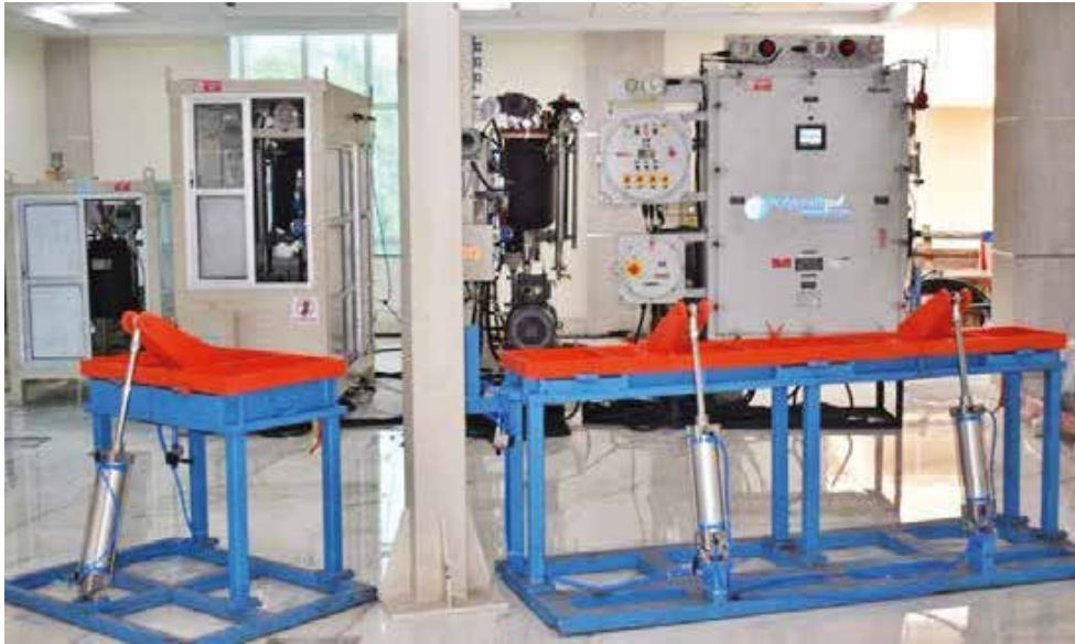
High Pressure PU Foam Processing Unit with Moulds established at Laboratory for Advanced Research in Polymeric Materials (LARPM) CIPET, Bhubaneswar
